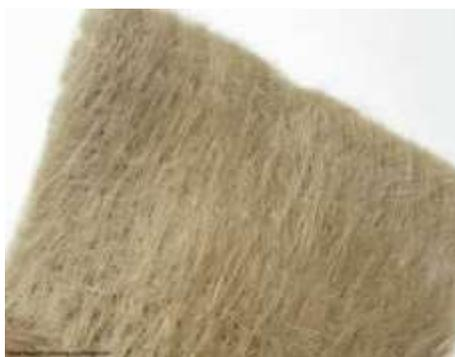
*Fig.2. Basalt fiber*
